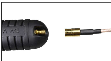
Each Probe offers a SMB-quick-connector...
