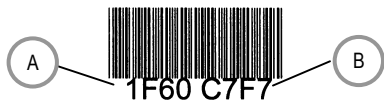
Figure 46: Sensing Head Calibration Data printed on the Cable (e.g. Head with two blocks of 4 numbers)
