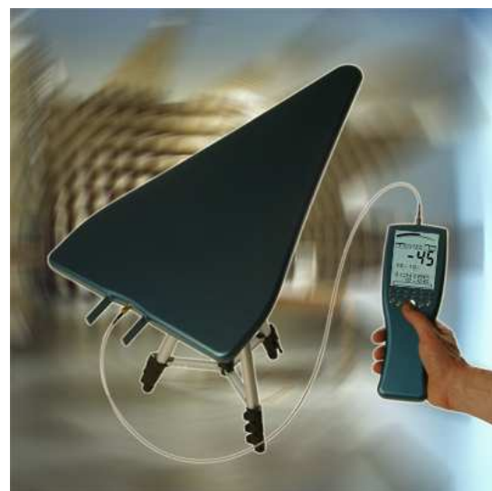
Spectrum Analyser and HyperLOG® directional antenna
