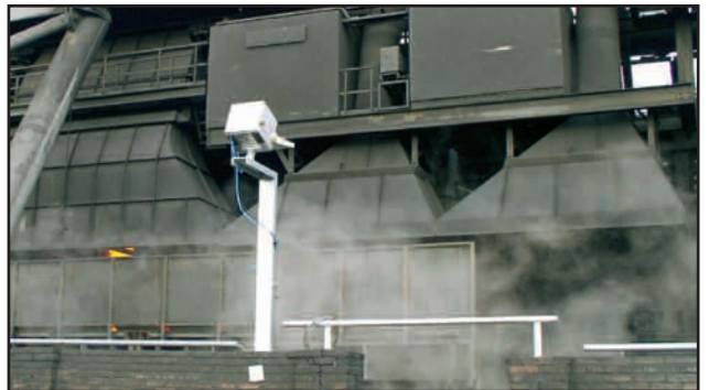
Automatic hot spot detection with an MP150 Linescanner increases safety during the coke process.
